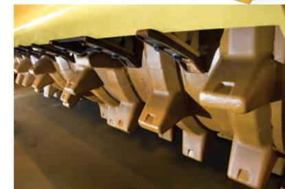
Two full width drums ensure uniform and efficient compaction
