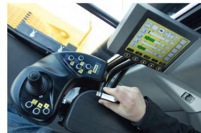
Command the compactor with easier controls and machine management with personalized USB key
